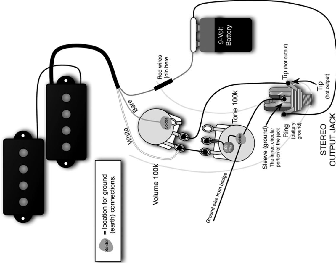
**Wiring Diagram for Pickup Models:**
