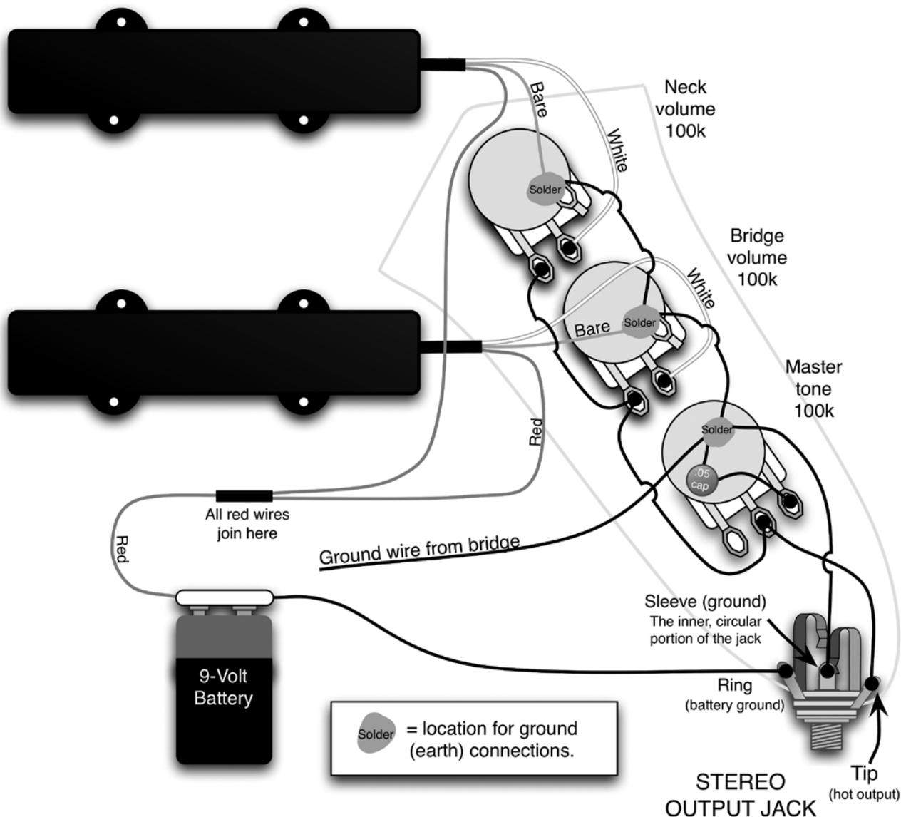
**Wiring Diagram for Pickup Models:**
