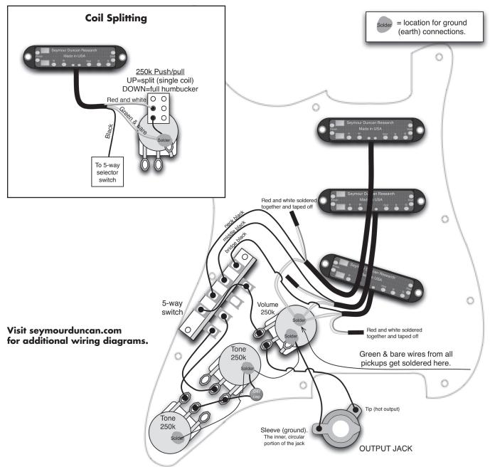
If two pickups sound thin and nasal when used together, chances are, they're out of phase with each other. If you're combining your Seymour Duncan pickup(s) with Fender® pickup(s) in the same guitar, you'll need to reverse the black and green wires on the Seymour Duncan. In other words, solder the black wire to ground and the green wire to the selector switch.
